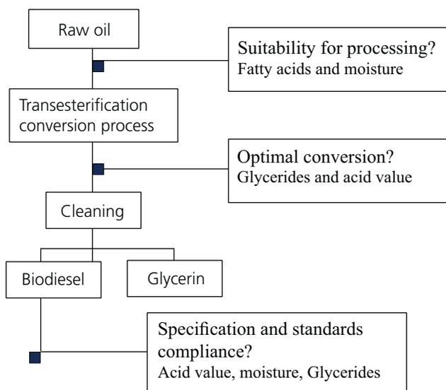
*Fig.1 Schematic description of the biodiesel production process and control points. The transesterification method is a popular way to make biodiesel because it requires only low temperature and pressure, the conversion rate is high and there is a direct conversion with no intermediate compounds*
