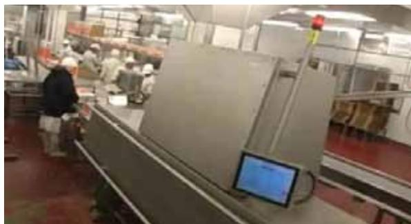
**Summary:** The MeatMaster is used for classifying each cardboard box according to its CL. This data is then used for creating more product ranges and tighter control. Also, foreign objects and metal are detected.
